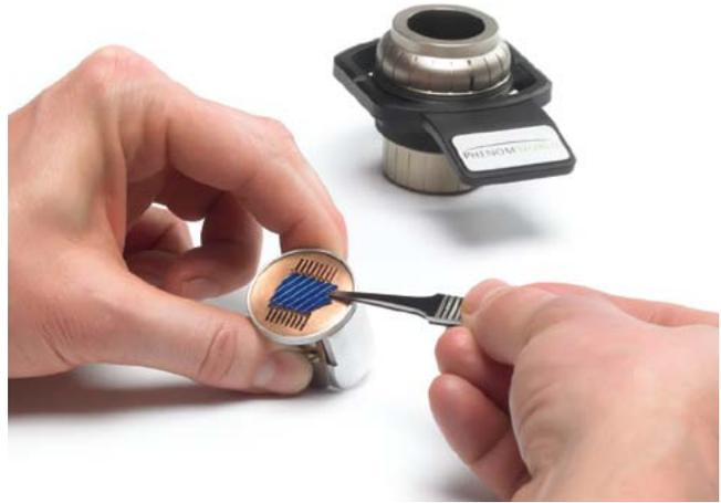
Sample preparation with micro-electronics insert.
