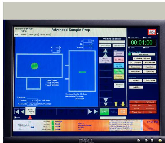
Highly interactive user control with a real-time representation of both the process parameters and the operating status.
